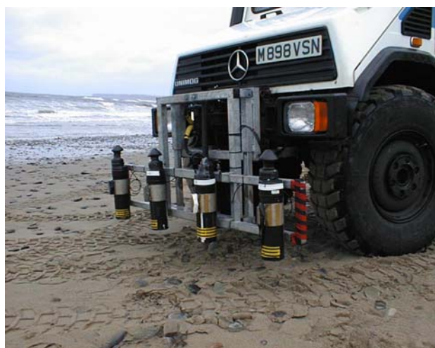
Figure 3 Groundhog Mrk 1 system, with four 76 x 76 mm diameter NaI(Tl) Detectors
